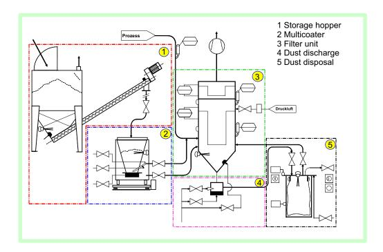
The storage hopper can be loaded at any time. A charge sensor gives a report, if the loading in the storage hopper goes below the minimum storage volume to guarantee the supply of the Multicoater with the precoat material. The charging level in the Multicoater is monitored by CNC in order to be refilled automatically.
